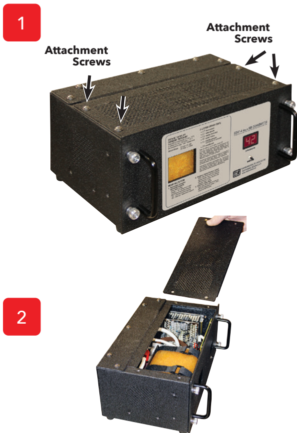
FIGURE 11. Desiccant Bottle Removal - Front Display Panel Mounting screws locations; open front panel
